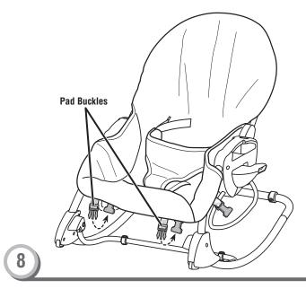
• Fasten the pad buckles on the front edge of the pad and underneath the seat. Make sure you hear a "snap" on both sides.
